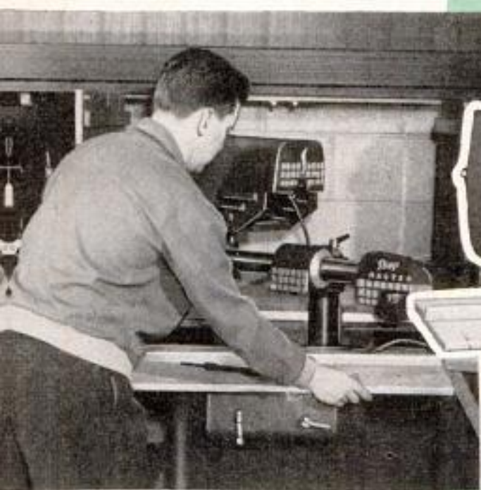
Photo above shows the combination tool being pulled from its niche in the wall cabinet. The two sets of double doors swing wide to provide clearance for the power tool. Photo at right shows tool in use within seconds of its removal from cabinet
